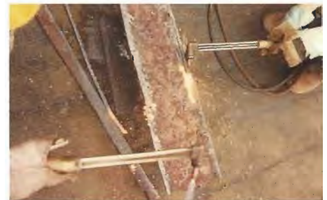
The end of the cut on the same plate, HGX using less oxygen has performed the cut faster, cleaner with less slag build-up than the Butane/Propane oxygen mixture.
