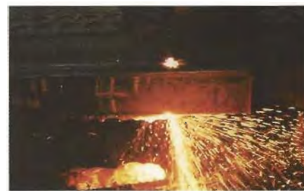
Automatic cutting of a 4" (10 cm.) bevel cut using an OXY/ HGX Fuel Gas mixture.
